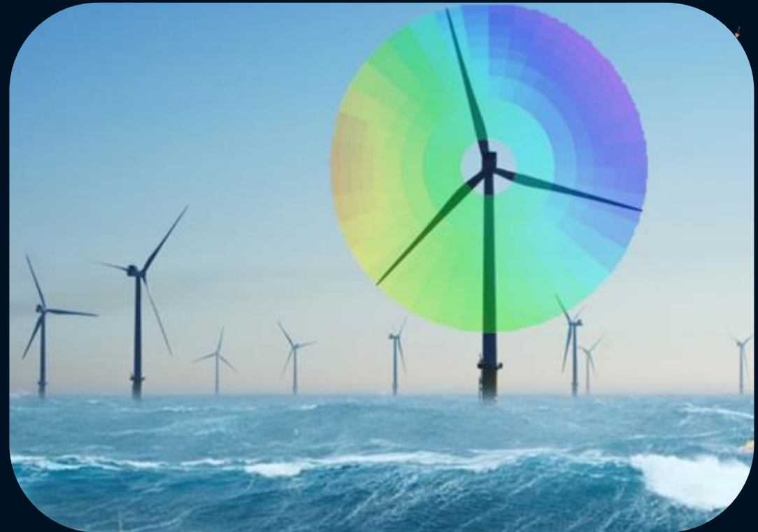
Heterogeneous inflow conditions at the rotor of an offshore turbine
