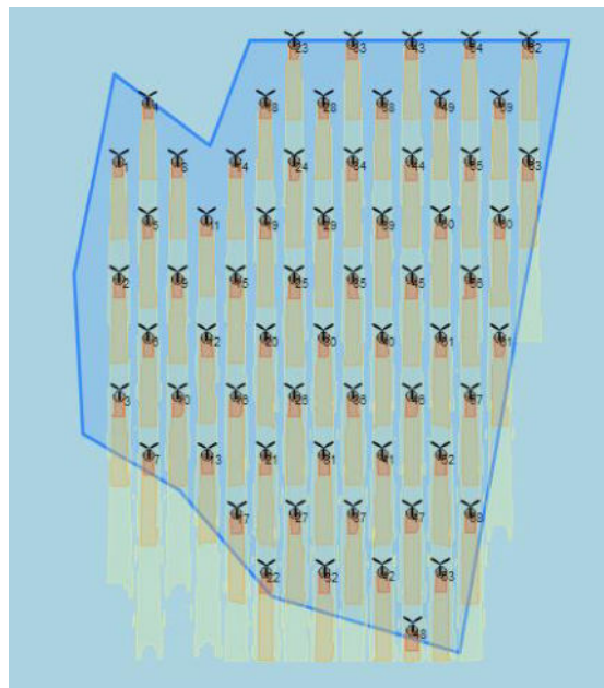
Figure 2.2.1.2: A wake simulation of the floating wind park with NOJ model (Jensen, 1983) in the dominant wind direction (North)
